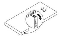
When there is an emergency to perform CPR on the patient, quickly pull the CPR valves to release air from mattress. The CPR valves are located at the head-end, right-hand-side of the mattress. The quick connector found from the pump unit can be disconnected for even faster deflation.
